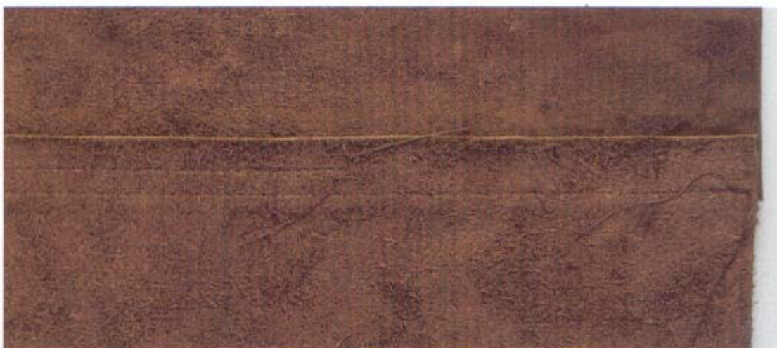
Photo 15 Method 2 lapped seam, wrong side
