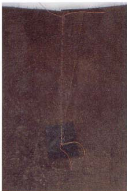
Photo 4. Lapped dart with reinforced point, wrong side
