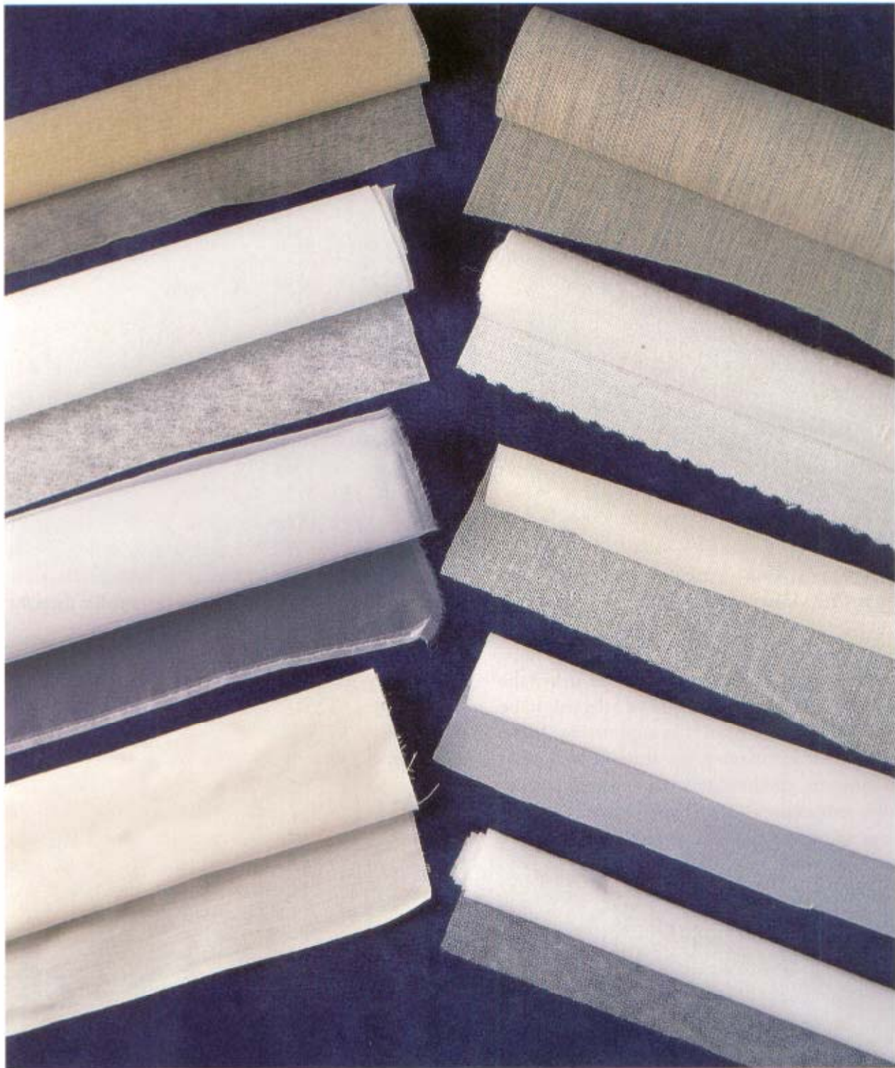
Interfacings suitable for leather and suede. Left, top to bottom: very lightweight nonwoven, medium weight nonwoven, organza, woven poly/cotton. Right, top to bottom: fusible hair canvas, woven poly/rayon, weft insertion, fusible tricot, low-temperature fusible.
