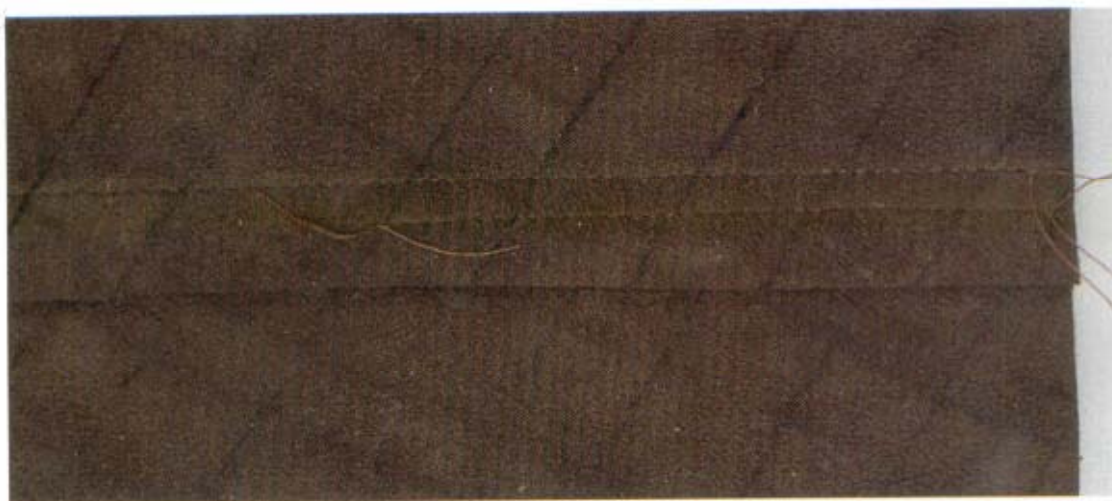
Photo 14 Method 1 lapped seam, wrong side
