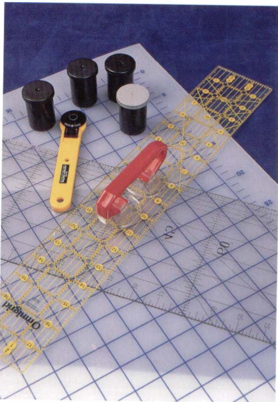
A rotary cutter and mat are the most efficient means of cutting leather and suede. Film canisters filled with sand make good pattern weights.
